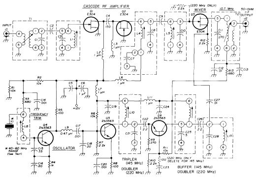
fig. 4. Schematic of vhf converter designed for use on two meters (values shown are for 145 to 155 MHz) and 220 MHz. Inductors and transformers are wound with no. 26 (0.4mm) wire. Tunedcircuit values may be changed as required for operation in adjacent commercial bands.
